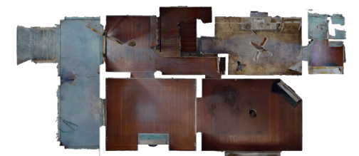
(Above) 3D LiDAR scan of existing building—first, second, and third floor plans and 3D view—used as the basis for drafting accurate existing building plans. (Opposite) Exterior view of existing house from Walnut Street, looking north.
