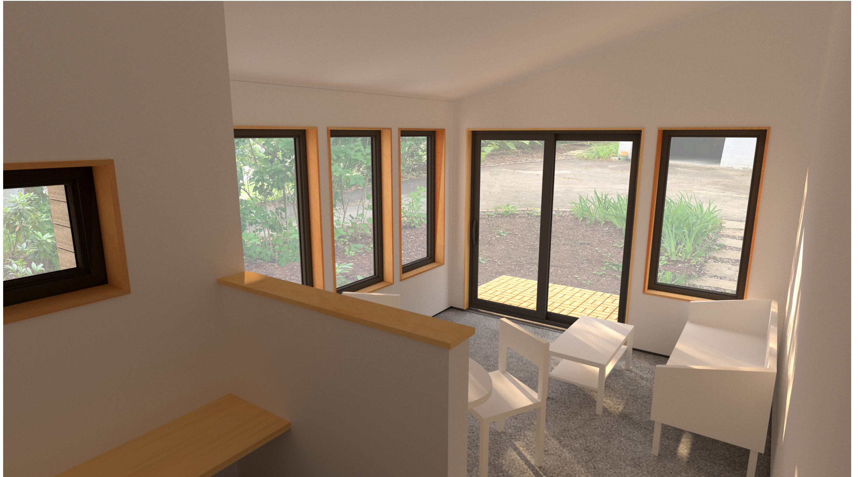
Interior rendering from proposed landing looking northwest. A small square window provides a peek to the rear entry walkway, giving the owners visual access to approaching visitors. In the lower sitting area, casement windows and a sliding door open the space up to the garden to the northwest while the solid wall to the east provides privacy and a sense of security.
