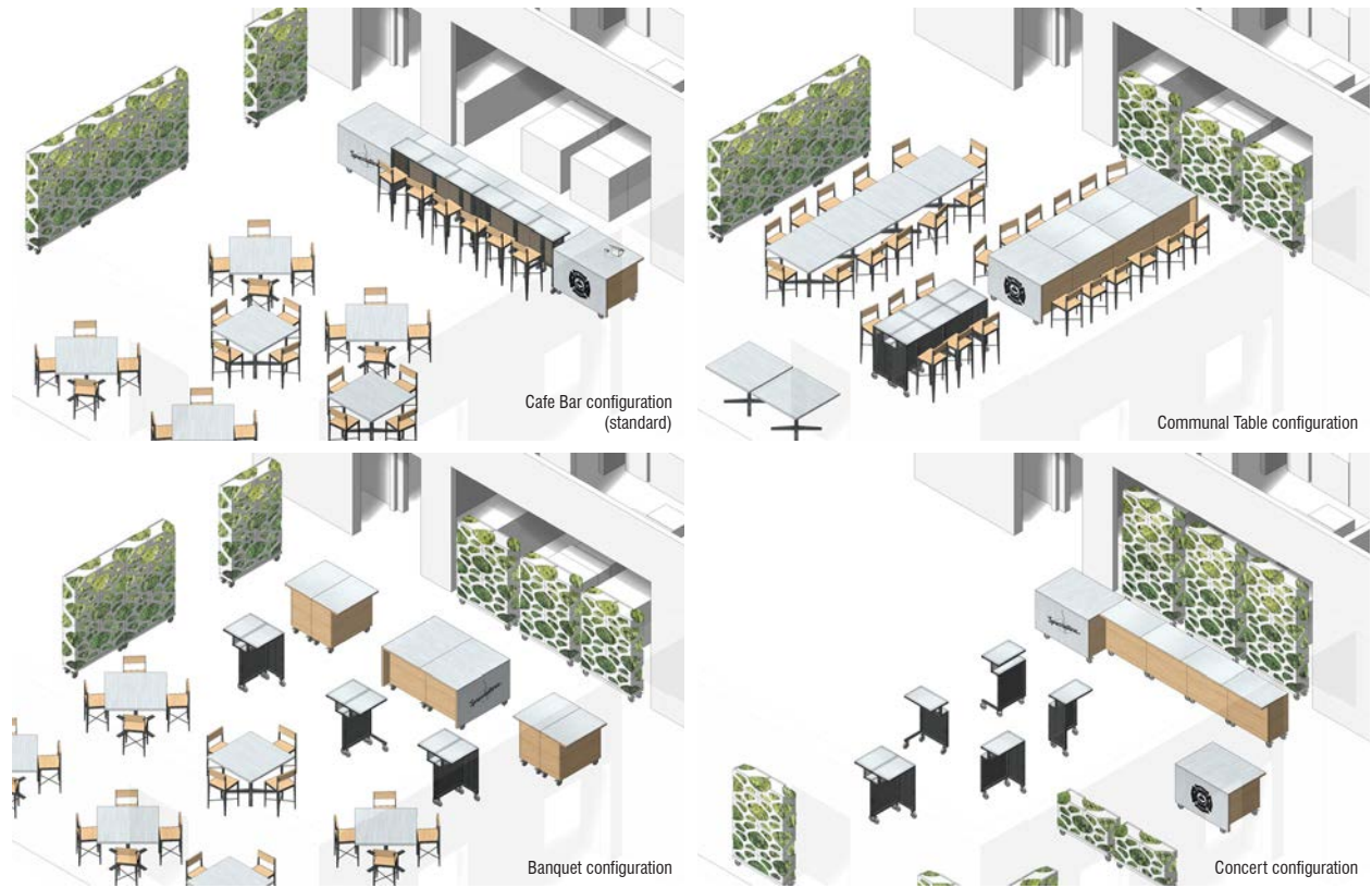
Design studies used to develop strategy for modularity/reconfigurability of the cafe elements.
