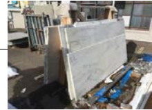
COUNTERTOP: Reclaimed marble slabs stored outside at building material reuse facility. The marble was cut to size and installed by apprentices as part of job skill training.
