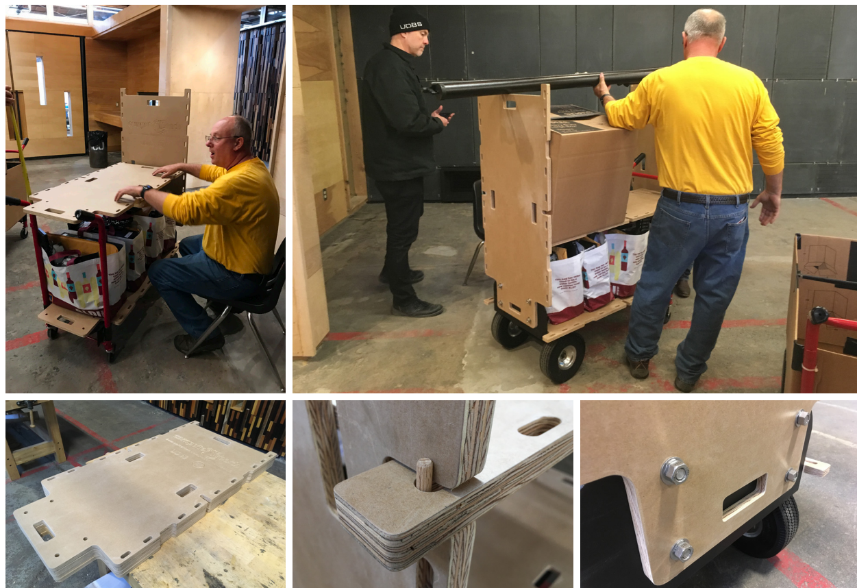
The REACH cart is the result of an iterative design, prototyping, and evaluation process directly involving the client. An initial prototype sought to create the cart from four universal panels that could be flat-packed when not in use. It proved difficult to incorporate the necessary functional, stability, and durability requirements into a single universal panel, however, and it was decided that a core box strategy would be explored instead.
