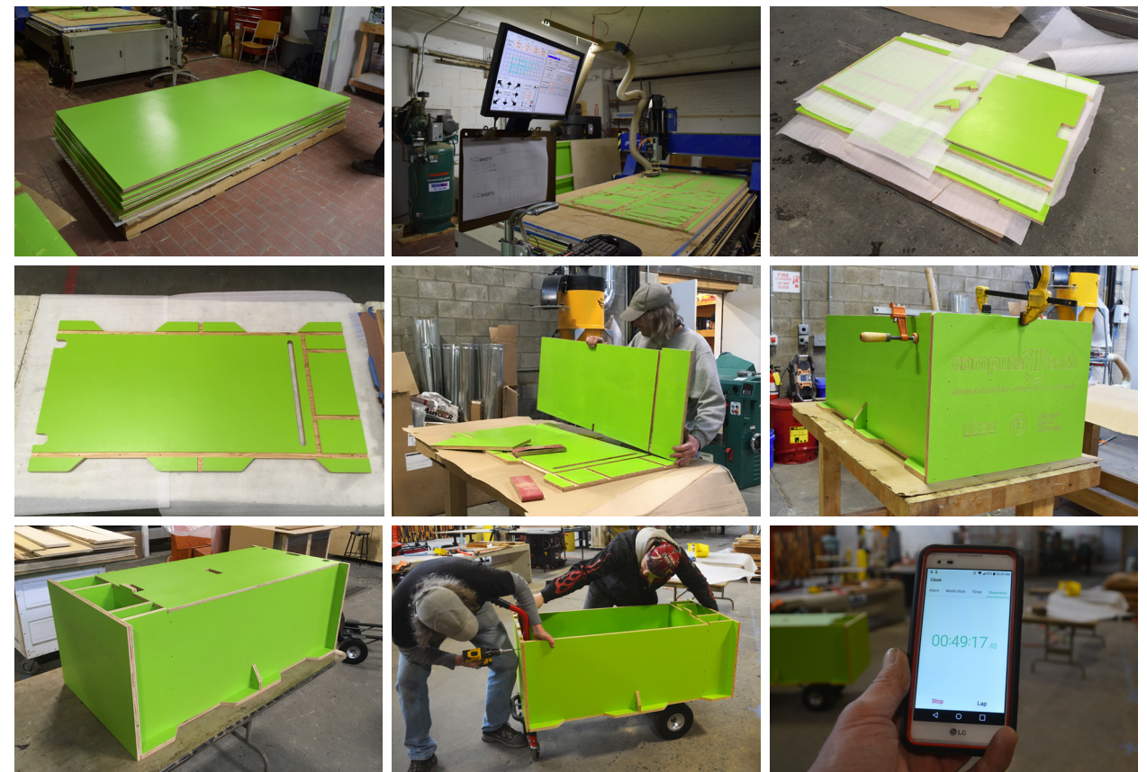
The REACH cart was designed for mass-production. Each cart is comprised of CNC-milled MDO panels that can be reproduced rapidly and with a high degree of mechanical precision. All dados, rabbets, and screw holes were routed into the panels by the CNC, allowing the carpenter to quickly align and assemble each cart. Each cart box can be assembled by one carpenter in under 50 minutes.
